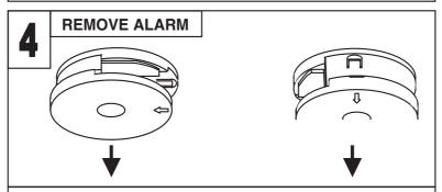
HOLD THE LOWER HALF OF THE ALARM AND REMOVE FROM THE BASE PLATE BY MOVING IT VERTICALLY DOWNWARDS, TOWARDS THE FLOOR.
